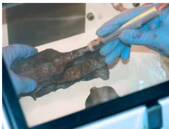
Figure 21. Cleaning with a micro-scale abrasion tester and glass bead.
