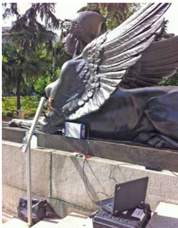
Figure 14. Electrochemical impedance spectroscopy (EIS) of the protective capacity of patinas and coatings on the sphinxes on the façade of National Archaeological Museum, Madrid.
