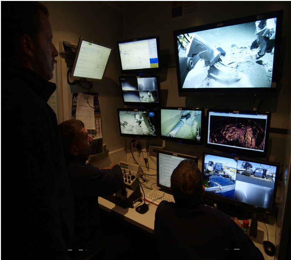
Figure 43: ROV control post.
