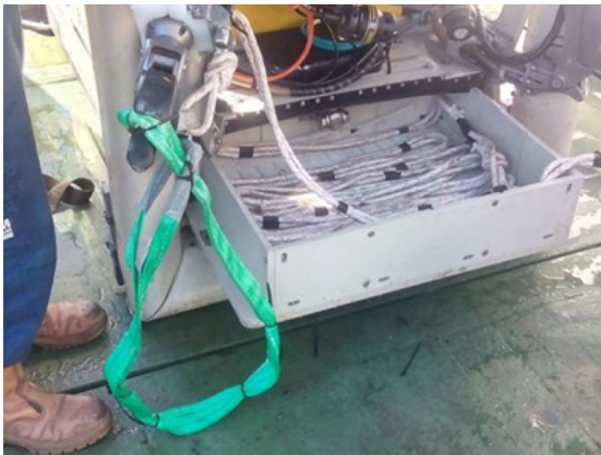
Figures 34 and 35: The ROV being prepared for DIVE03: a rope in the sample container, one end with a loop prepared in the right arm of the ROV and the other end of the rope in the left arm. The red buoy helps locate this end.
